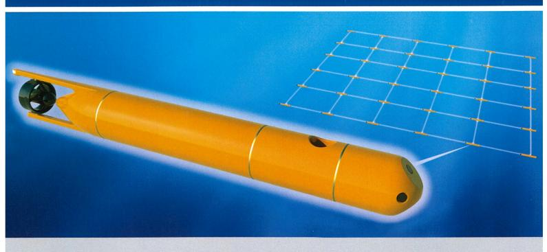
Autonomous Unmanned Underwater Vehicle fitted with a seismic signal receiver is designed for operations in hard—to—reach water areas of freezing seas with severe ice and metocean conditions.
